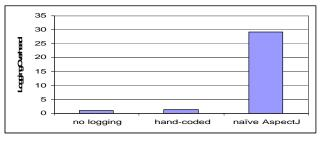
Figure 4. Overhead with logging disabled
